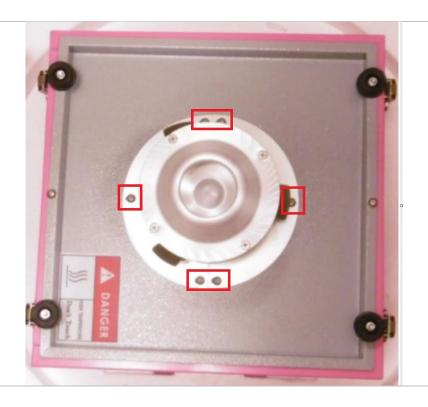
**STEP 2:** Unscrew 1 bolt which is located behind the cover - on the moving element (the spindle)
