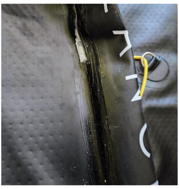
AIR LEAKAGE IN PADDLE BOARD - information and visualization of what is not repairable in service
