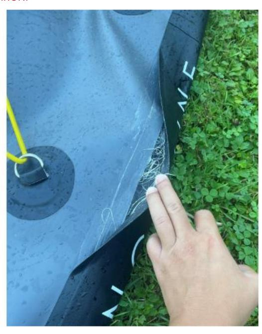
AIR LEAKAGE IN PADDLE BOARD - information and visualization of what is not repairable in service
