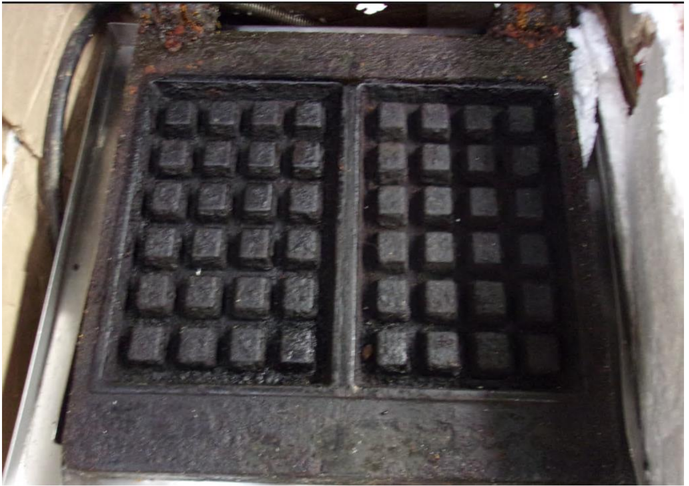
SURFACE OF HEATING PLATE– visualization of not cleaned & maintenance surface [out of warranty]
