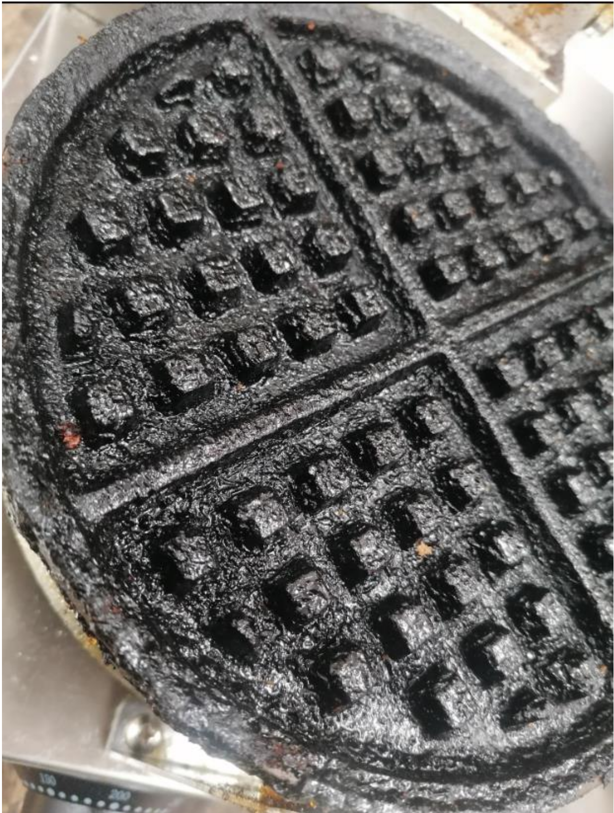
SURFACE OF HEATING PLATE– visualization of not cleaned & maintenance surface [out of warranty]
