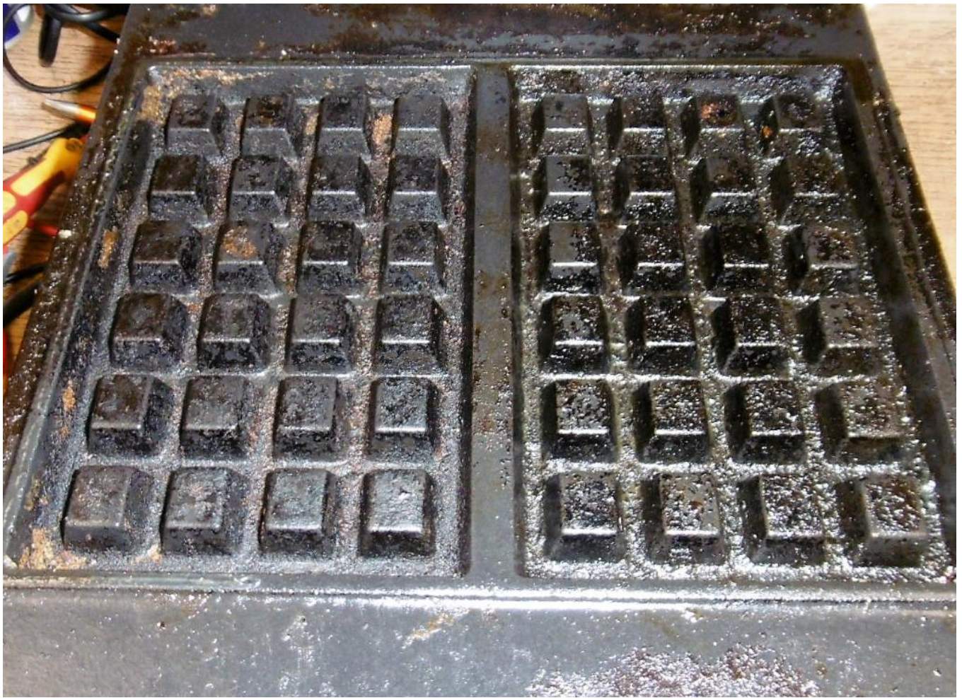
SURFACE OF HEATING PLATE– visualization of not cleaned & maintenance surface [out of warranty]
