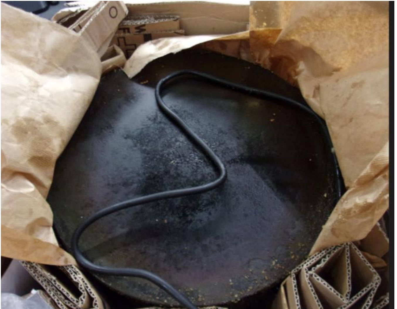
SURFACE OF HEATING PLATE– visualization of not cleaned & maintenance surface [out of warranty]
